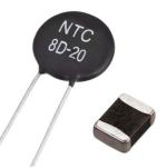
resistance are called PTC (Positive Temperature Coefficient) thermistors. NTC thermistors are often made of metal oxide powders which are compressed and sintered at a high temperature. The materials used include  $Mn_2O_3$ , NiO,  $Cr_2O_3$ , CuO,  $Fe_2O_3$ , TiO<sub>2</sub>, etc. They can also be made of semiconductors with different levels of doping.
