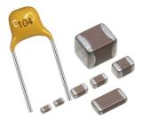
Through-hole ceramic capacitors form a component in the shape of disc, "droplet" or otherwise shaped component (it can be highly diverse and non-standard depending on the manufacturer) with wired leads. The characteristic features of through-hole capacitors include high values of the maximum operating voltage, but relatively low capacitance values.
