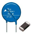
Varistors are useful for short term protection in the case of high transient voltages (on the order of 1-1000 microseconds). However, they are not suitable for coping with sustained surges. If the pulse energy, measured in Joules (J), significantly exceeds the absolute maximum strength values of the varistor, it will cause damage to it. The most important types of varistors are:
