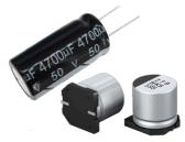
These capacitors have a large capacitance (from 1  $\mu$ F upwards) but have poor properties in the higher frequency ranges and are not usually used in circuits above 100KHz. In addition, the shortcomings include high leakage currents, lower tolerance, and limited service life. As standard, the ESR resistance is quite high, while the manufacturers' offer includes a special type of aluminium capacitors marked as Low ESR – i.e., with low ESR resistance.
