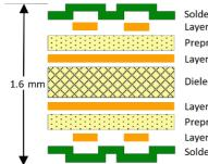
Solder mask, thickness 20 um Layer 1 (TOP), copper thickness 35 um Prepreg, thickness 200 µm Layer 2, cooper thickness 35 Dielectric, thickness 1000 µm Layer 3, copper thickness 35 µm Prepreg, thickness 200 µm Layer 4 (BOTTOM), copper thickness 35 µm Solder mask, thickness 20 um
