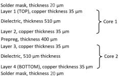
A type I multilayer printed circuit board consists of one core and two additional layers of copper. With this design, holes can only be made between layers 1-2-3-4 (through) and 2-3 (buried). This is the most common variant of four-layer boards and at the same time the cheapest.
