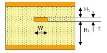
$$Z_0 = \left[\frac{80}{\sqrt{\varepsilon_r}}\right] \times \ln\left[\frac{1,9(2H_1+T)}{0,8W+T} \times (1 - \frac{H_1}{4H_2})\right], \text{ [ohm]}$$
