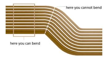
Copper conductors on the flexible printed circuit board should change direction smoothly (you have to avoid sharp angles), the same applies to changes in the width of the conductors - the transition from a wider conductor to a narrow one must be gradual:
