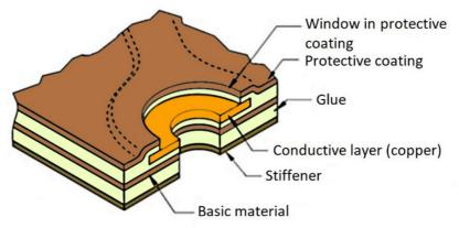
The most common base material for flexible circuit boards is polyimide. Although PET is cheaper, manufacturers use it much less frequently due to its lower heat resistance. On the other hand, PET has advantages in terms of chemical resistance and moisture absorption. One-sided flexible circuits for automotive industry are most often produced from PET.
